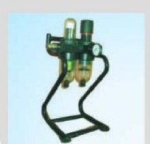
Low Pressure Conditioner Item Code 13097 Regulator, PC Bowl, Coalescing + Borosilicate 0.3 micron Particulate + GAC odour filter, Gauge and manual drain. Inlet Ø 6mm
